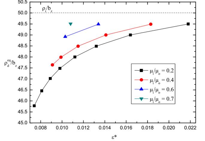
FIG. 2. (Color online)  $\rho_d^{eq}/b_z$  versus  $\epsilon^*$  for different values of  $\mu_i$ , with  $\mu_o=100$  GPa,  $\nu_i=\nu_o=0.3$ ,  $r_i=50b_z$ , and  $r_o=65b_z$ .
