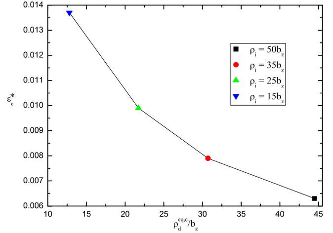
FIG. 5. (Color online)  $\epsilon_c^*$  versus  $\rho_d^{eq,c}/b_z$  for different values of  $\rho_i$  and  $\rho_o$ , with  $\rho_o - \rho_i = 15b_z$ ,  $\nu_i = \nu_o = 0.3$ ,  $\mu_i = 10$  GPa, and  $\mu_o = 100$  GPa.
