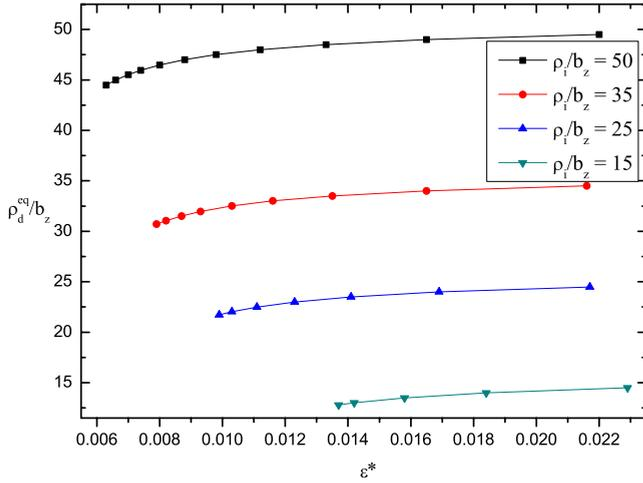
FIG. 4. (Color online)  $\rho_d^{eq}/b_z$  versus  $\epsilon_c^*$  for different values of  $\rho_i$  and  $\rho_o$ , with  $\rho_o - \rho_i = 15b_z$ ,  $\nu_i = \nu_o = 0.3$ ,  $\mu_i = 10$  GPa, and  $\mu_o = 100$  GPa.
